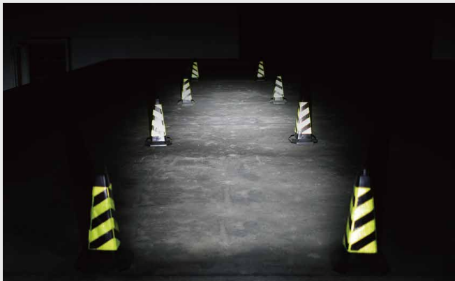
Hammer E170 Plus (low beam:150lux)
